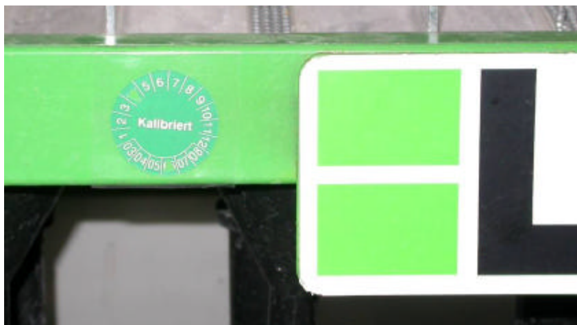
Fig 3: badge "Kalibriert" that shows the duration of inspection validity. In this case next inspection in April 2006
