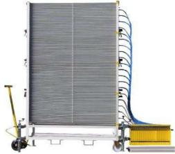
The sprayer must have placed for the test patternator that at least 80% of the sprayed fluid is caught. Emptying the measuring glasses must as such way that it is able take to bring the spayed liquid back in the tank.
